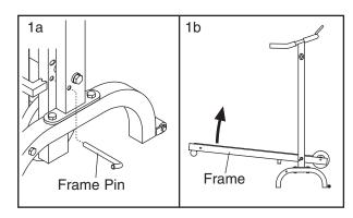
2. Using your right hand, pull the latch knob to the right and hold it. Raise the frame until the hole in the frame is aligned with the latch pin. Then, slowly release the latch knob. Make sure that the
